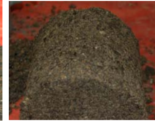
Sand Soil 25% Topsoil 3/8" 15% Compost 60% Coarse Sand
