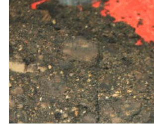
Tree Soil 60% Topsoil 2" 15% Compost 25% Coarse Sand
