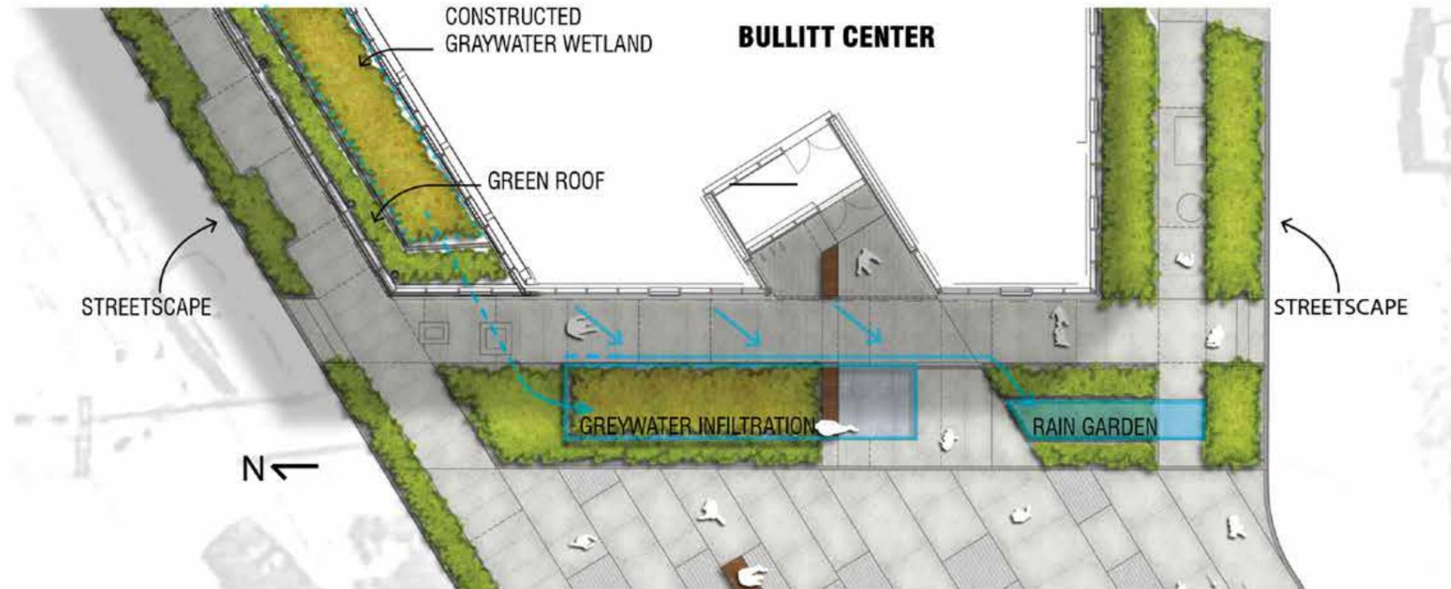
Rooftop rainwater is collected and used in the building for potable uses. Greywater flows to constructed wetlands to be treated and infiltrated through planters at grade. Stormwater flows to the rain garden. Permeable grating allows both function and access.
