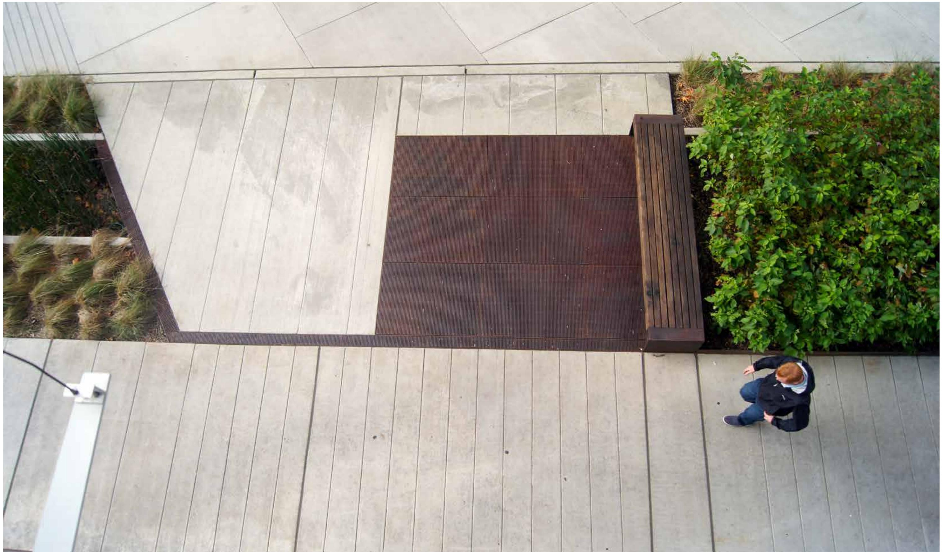
Detail view of 15th Avenue's curbless streetscape where a greywater planter, bench, grating, and trench drain bypass toward the rain garden and various planting typologies, all visible to the public.
